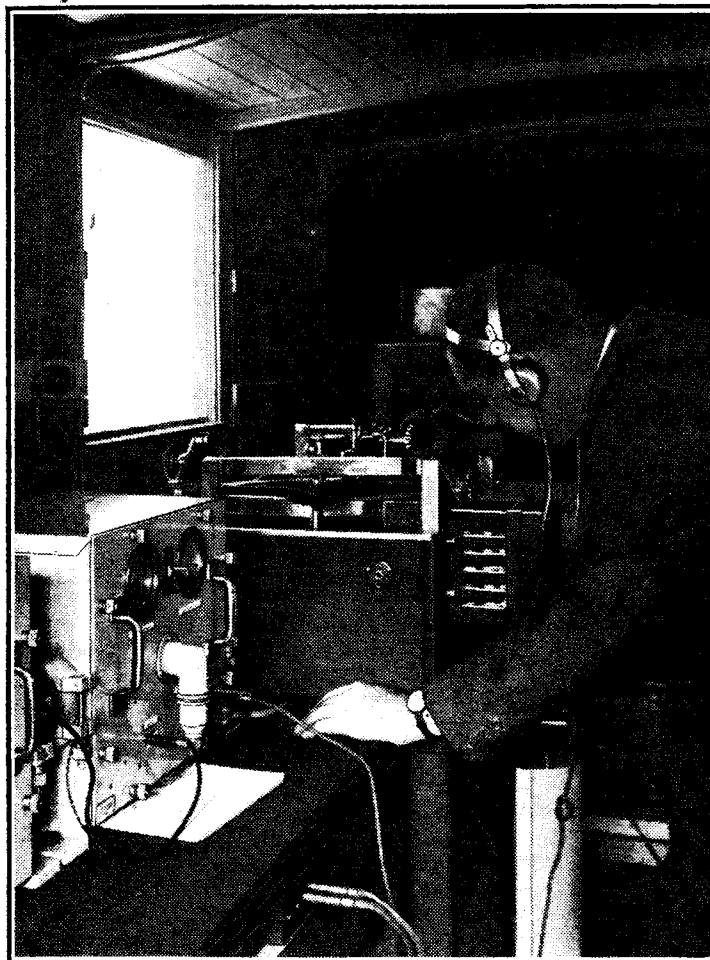
The "sound-on-disc" principle has been adopted for the B.B.C.'s mobile recording unit.
